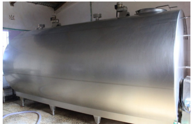
Figure 26: Milk Cooling Tank at Muhotetu Dairy Farmers Co-operative Society cooling plant (Day 3)
